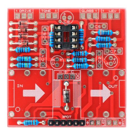
First of all place the IC sockets (without the ICs). Pay attention to the orientation! The small notch in the socket should be oriented as indicated in the PCB.
